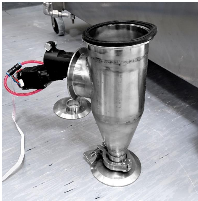
Figure 2: CPS1 - mechanical interface with 3D-printed prototype.
