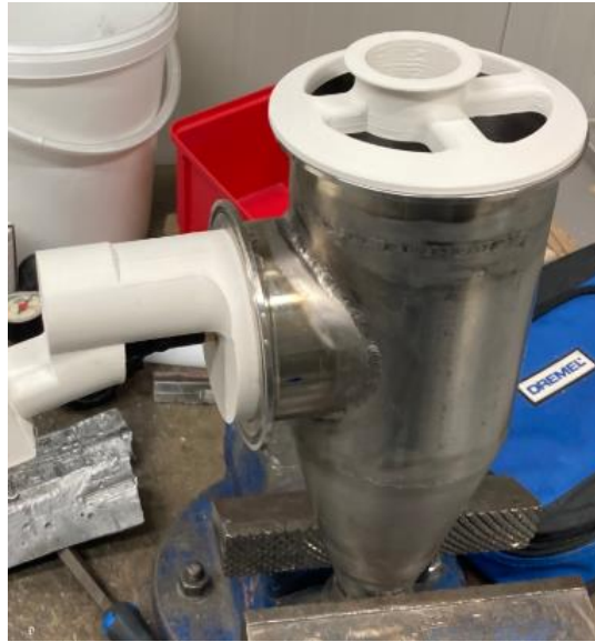
Figure 10 Metal cylinder to hold the Raman or Parsum probe
