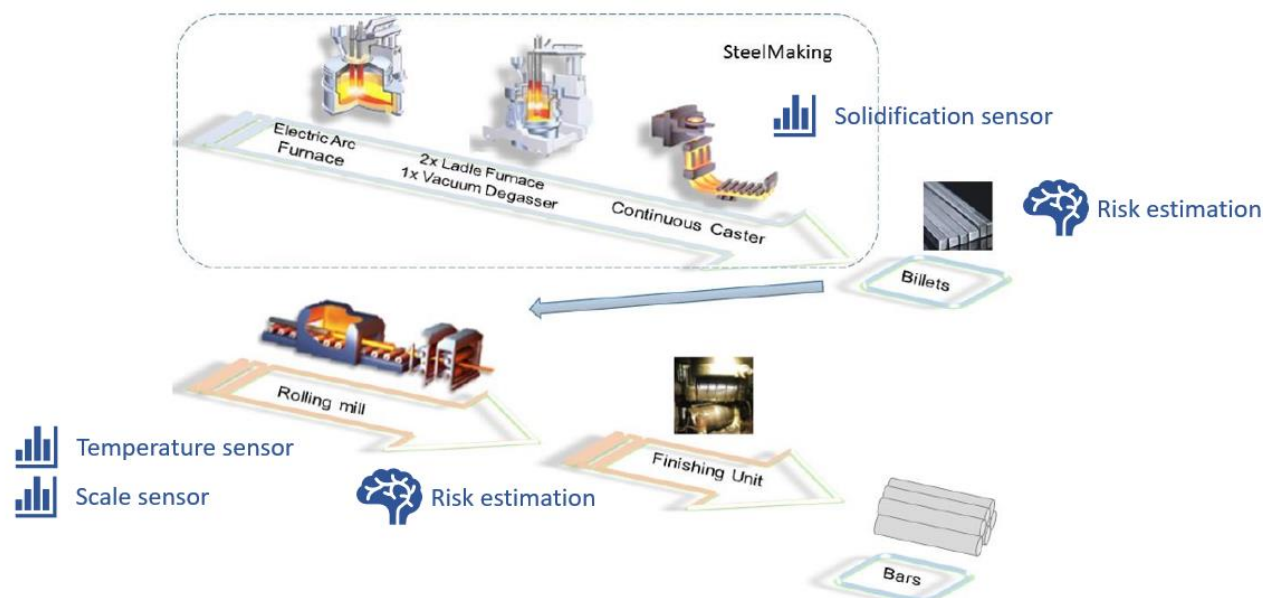
Figure 3: Overview of the steel production chain, with the position of the solidification (CSS2), temperature (CSS3) and scale sensors (CSS4), as well as the two risk estimators.
