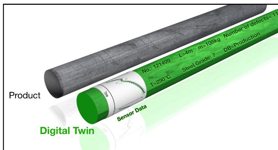
Figure 2: A digital twin of a steel long product
