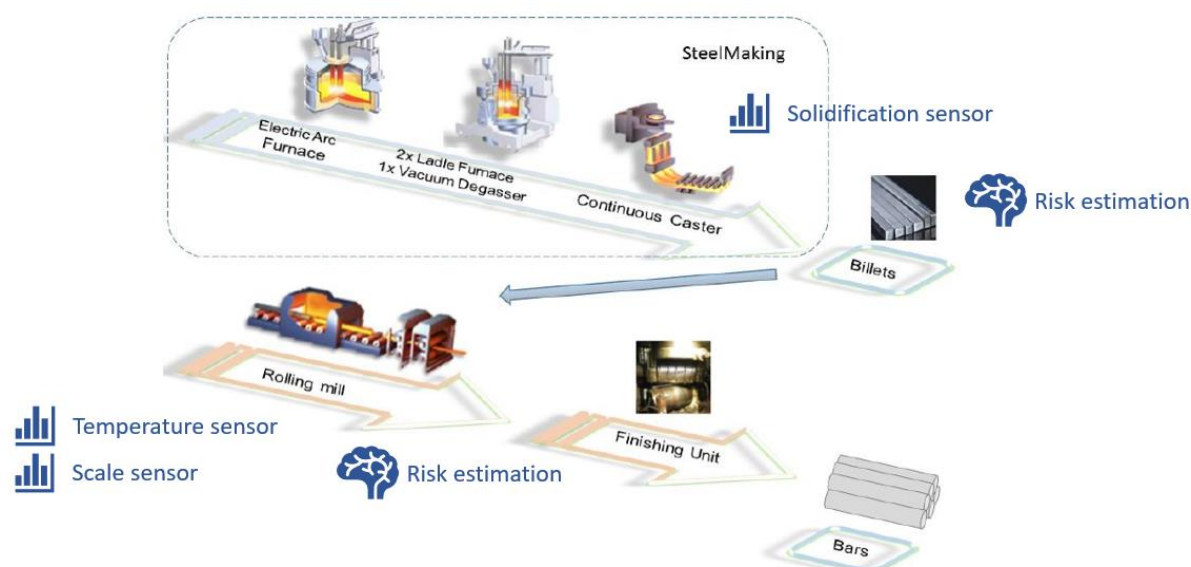
Figure 2: Steel processing chain with the logical position of the two risk estimators.
