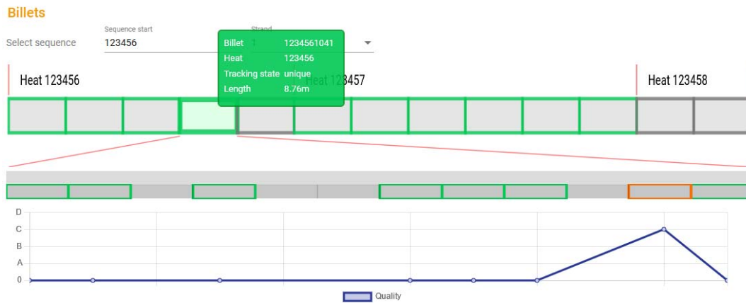
Figure 7: Visualization of billet and bar twins in the steel use case. Rectangles in the upper row represent billets (steel semi-products) and those in the middle row represent bars (the final products) made from a single billet. Colors indicate the tracking status (green: successful, grey: missed, orange: duplicate).
