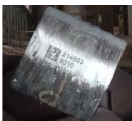
Figure 6: A marked steel billet.
